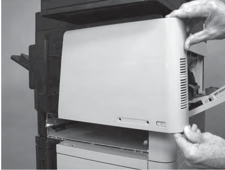
Figure 1-477 Remove the cover
