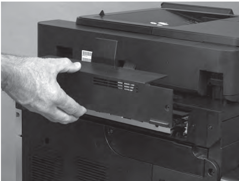
Figure 1-398 Install the cover
