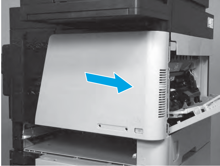
Figure 1-823 Slide the cover to the right
