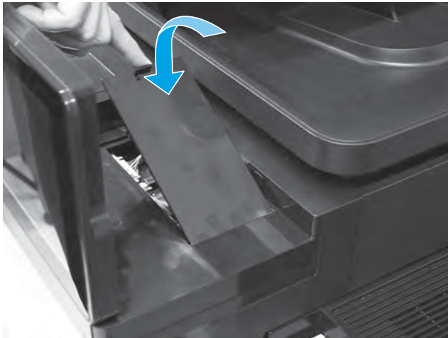
Figure 1-173 Install the cover
