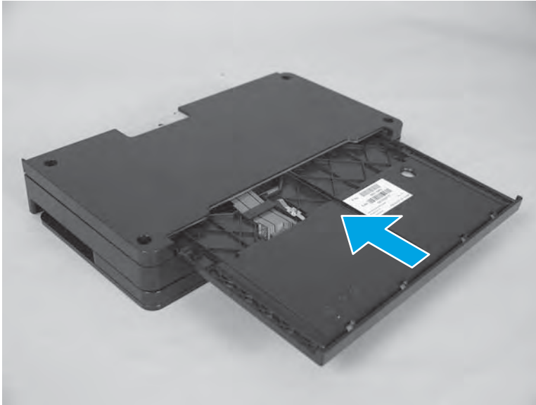
Figure 1-131 Slide the keyboard tray in
