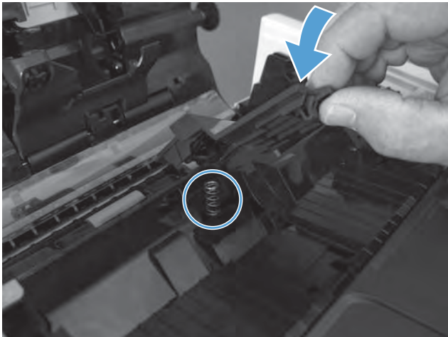
Figure 1-212 Position the separation pad on the product
