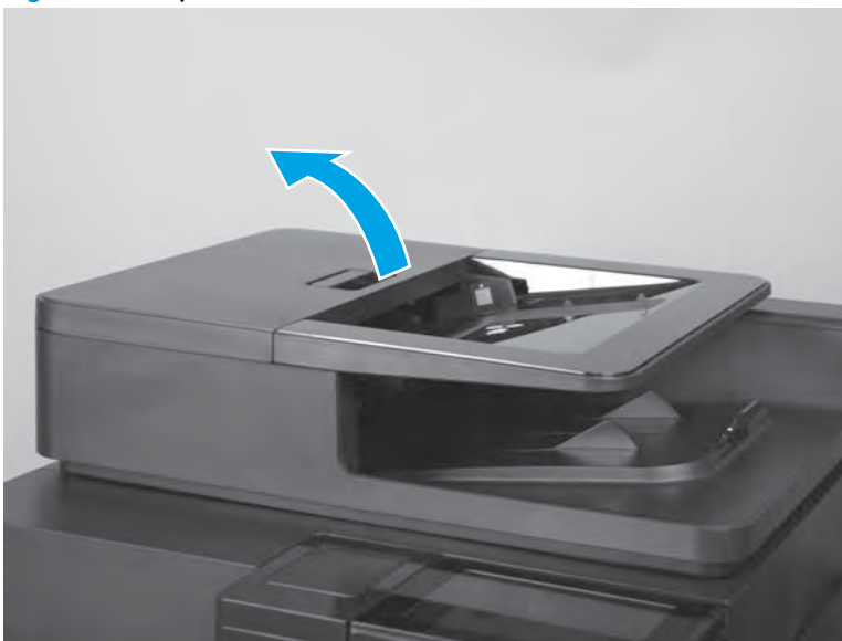
Figure 1-16 Open the document-feeder door
