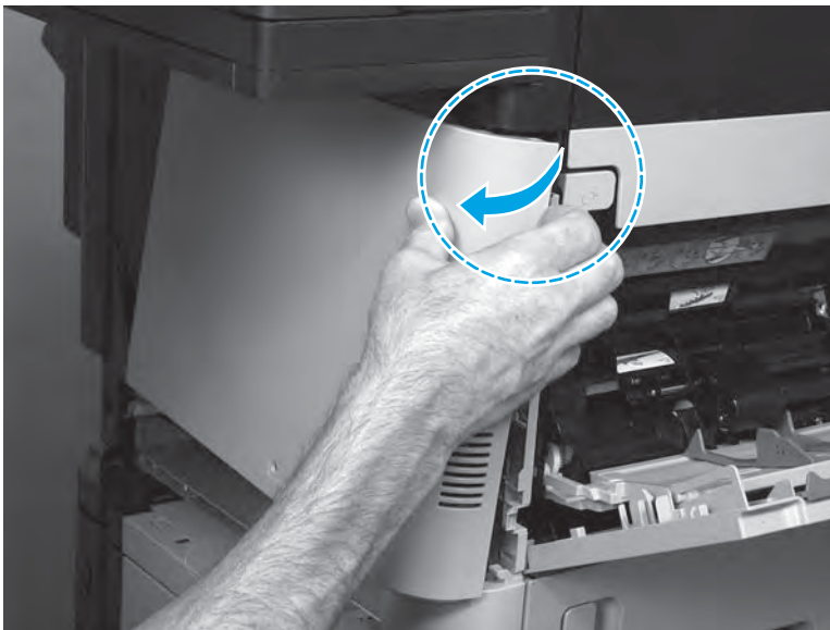
Figure 1-822 Release the right-upper corner
