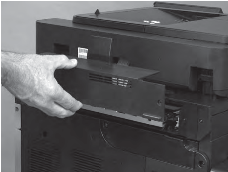
Figure 1-258 Remove the cover
