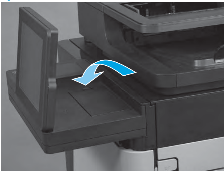
Figure 1-143 Install the cover
