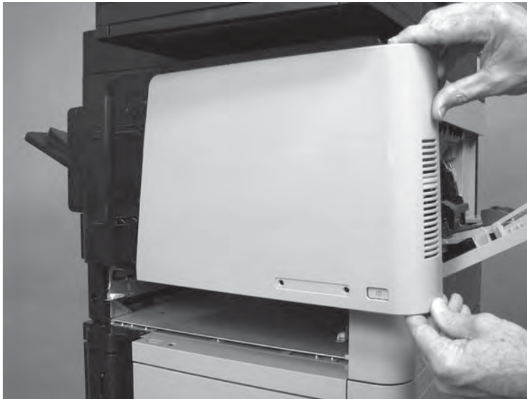
Figure 1-824 Remove the cover
