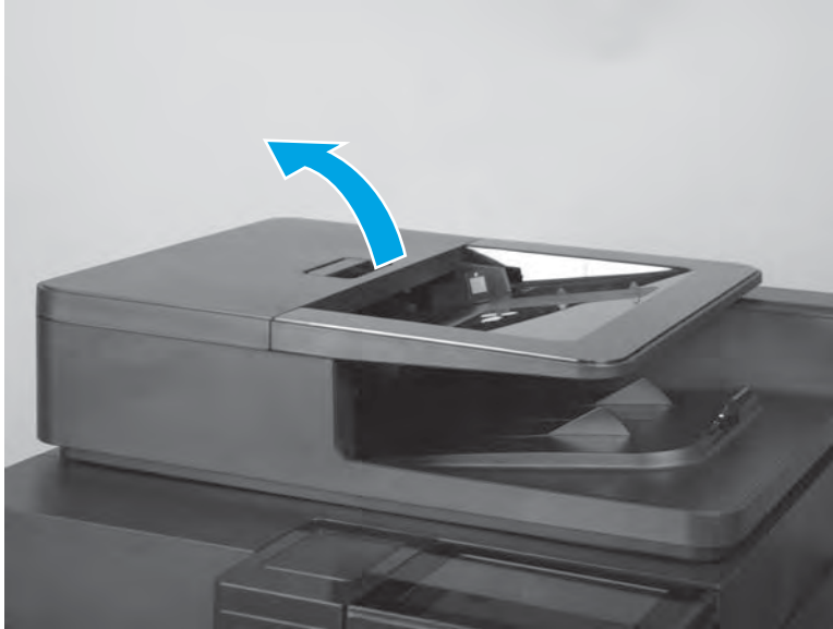
Figure 1-206 Open the document-feeder door
