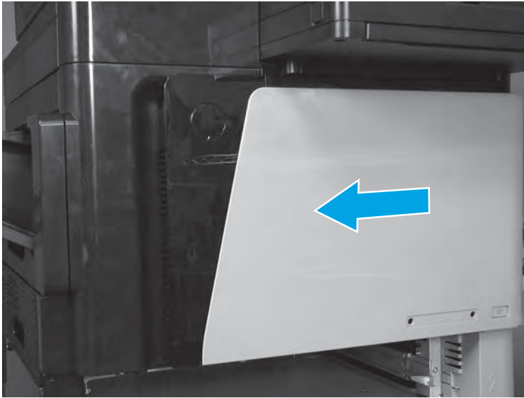
Figure 1-482 Slide the cover to the left
