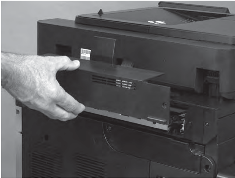
Figure 1-254 Remove the cover
