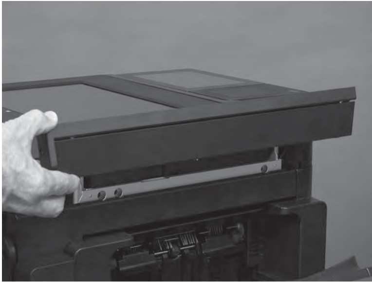
Figure 1-364 Remove the cover
