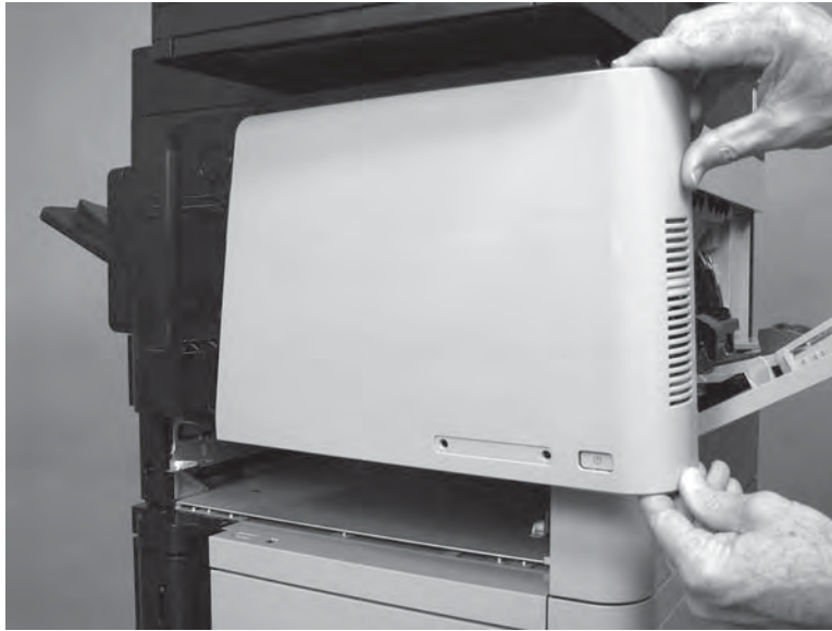
Figure 1-418 Remove the cover
