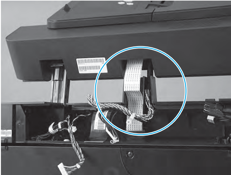
Figure 1-305 Route the document feeder FFC and cables
