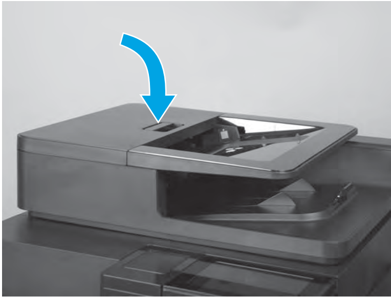
Figure 1-239 Close the document feeder cover
