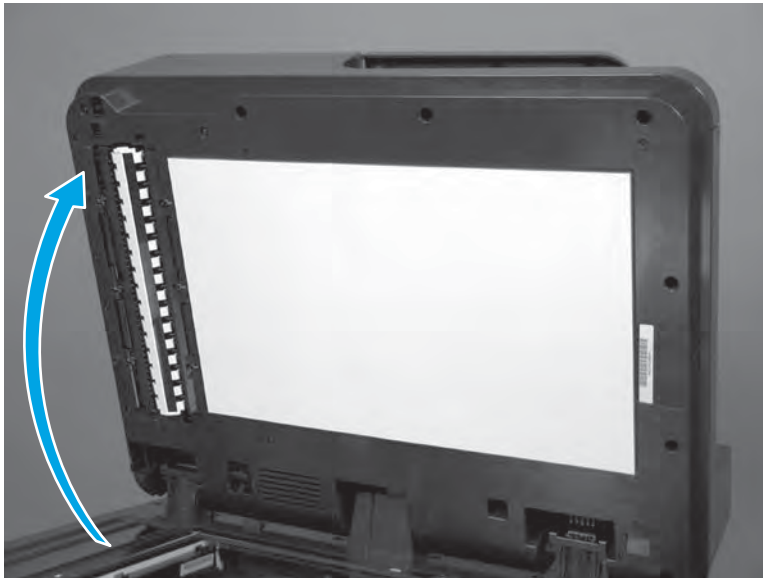
Figure 1-219 Open the document feeder
