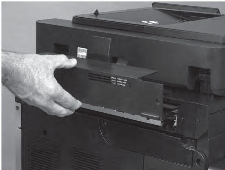
Figure 1-283 Install the cover
