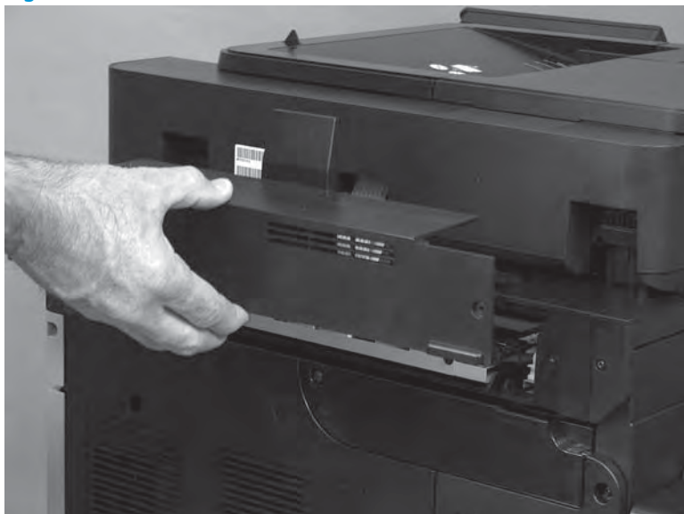
Figure 1-337 Remove the cover
