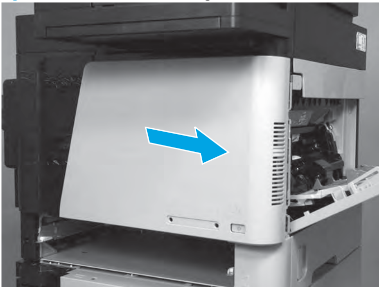
Figure 1-476 Slide the cover to the right
